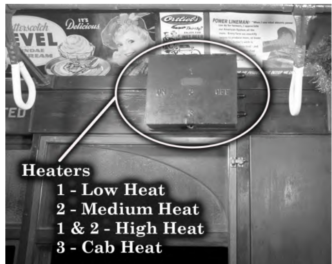
66 - Heater Switch Box
